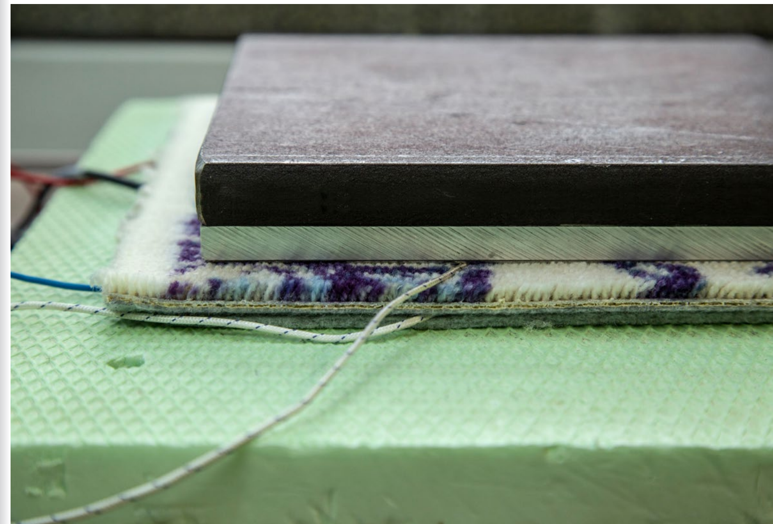
Fig. 57: test setup for thermal resistance
