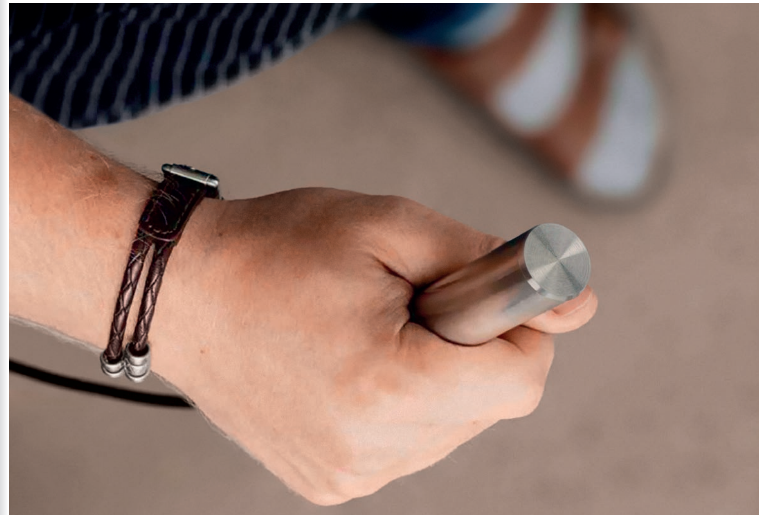
Fig. 63: walk-on test on floor covering with hand electrode; source: TFI AAachen
