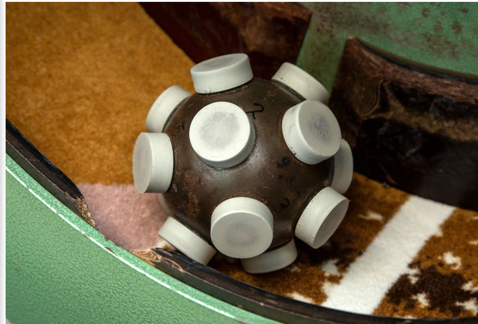
Fig. 43: steel ball with rubber stamps in Vettermann drum
